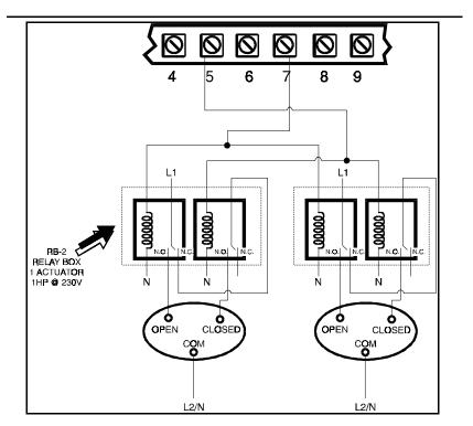
Fig 4a Two actuators connected on the same output
